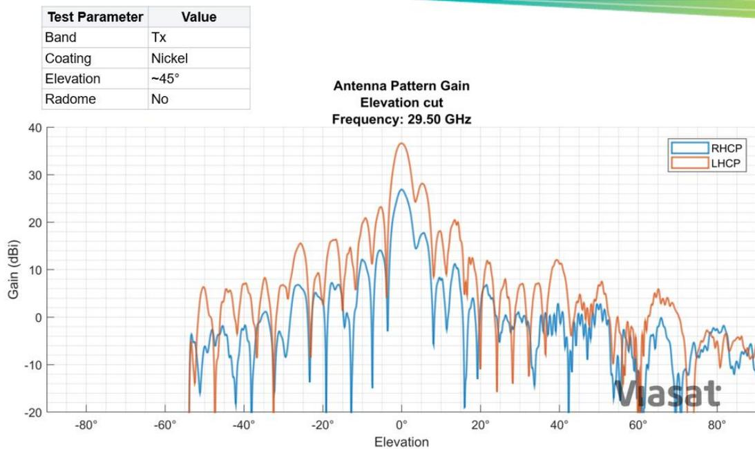
**Figure 45 - Antenna Pattern Gain at 29.5 GHz - Elevation cut at 45 degree elevation**
