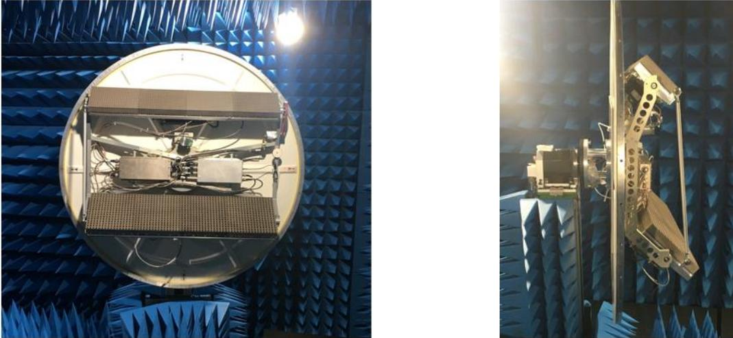
Figure 40 - Antenna pattern test setup
