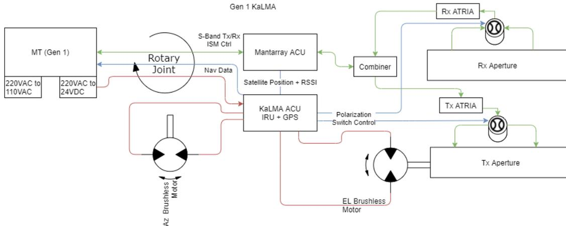
**Figure 23 - Architecture diagram of the KaLMA antenna**
