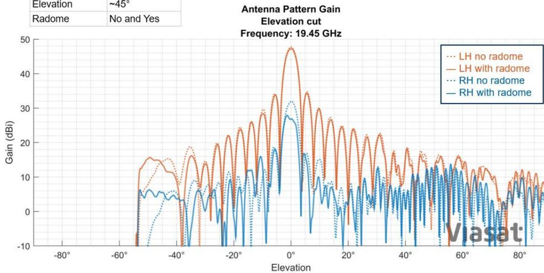
**Figure 49 - Evaluation of the effect of the radome on the Antenna Pattern Gain – Elevation cut at 19.45 GHz**
