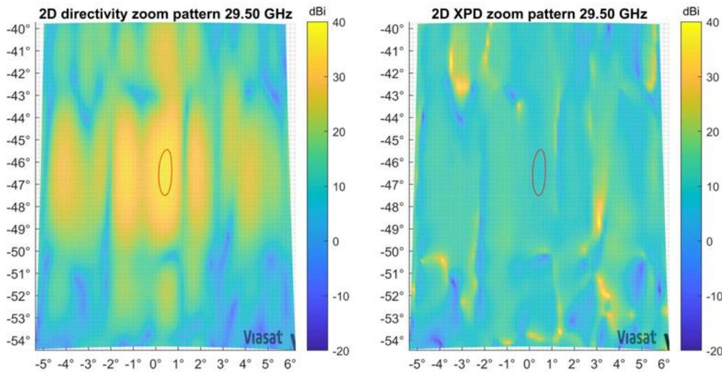
**Figure 55 - Antenna pattern main beam detail at 29.5 GHz at 45 degree elevation**
