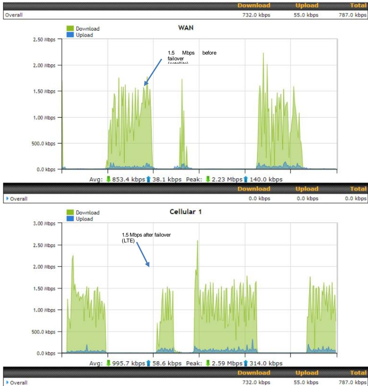
**Figure 73 - Data rates on the satellite and LTE link**
