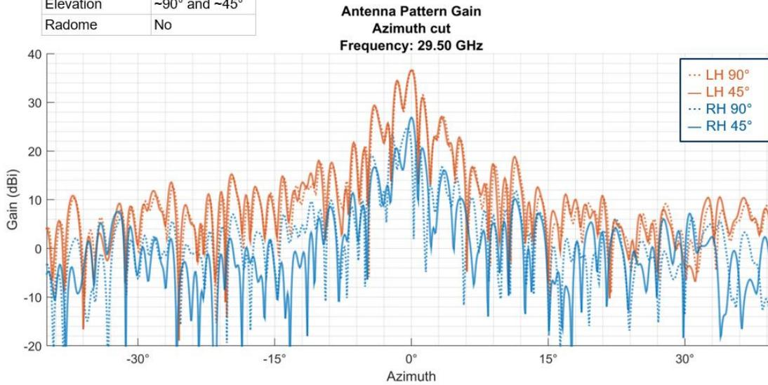
**Figure 50 - Comparison of the Antenna Pattern Gain - Azimuth cut at elevation of 45 and 90 degrees at 29.5 GHz**
