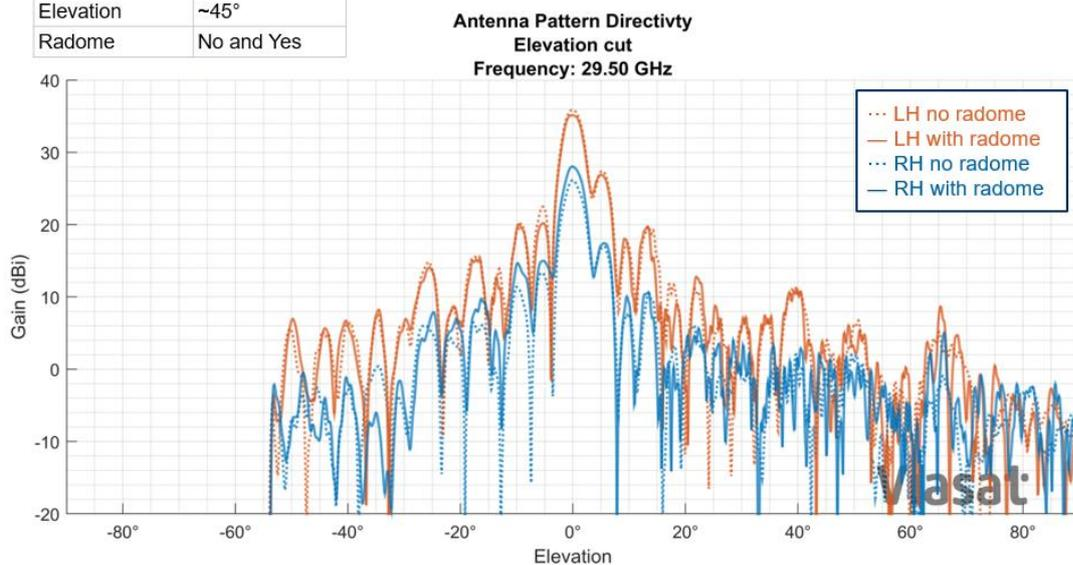
**Figure 53 - Evaluation of the effect of the radome on the Antenna Pattern Gain - Elevation cut at 29.5 GHz**
