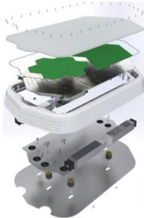
**Figure 36 - Phased antenna array for land mobile applications - exploded view. The total height of the terminal is below 11cm, but it can go even lower for the future designs.**
