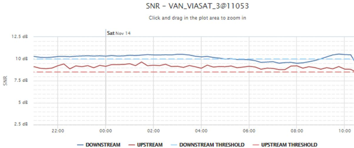
**Figure 74 - SNR on the upstream and downstream link on the KaLMA**
