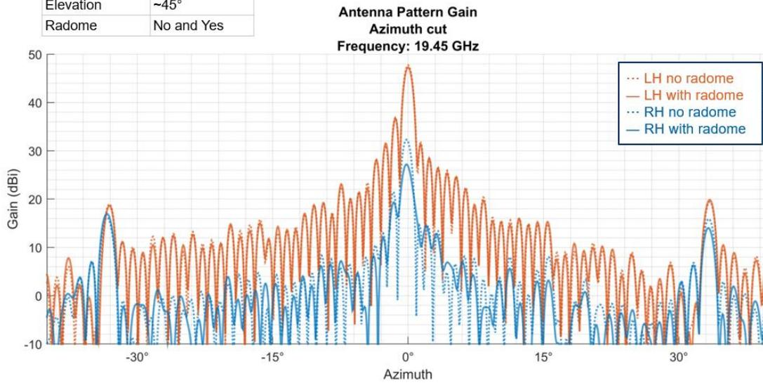
**Figure 48 - Evaluation of the effect of the radome on the Antenna Pattern Gain - Azimuth cut at 19.45 GHz**
