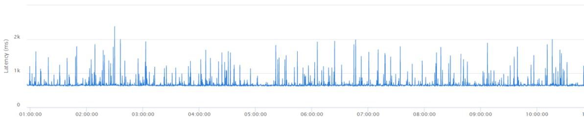
**Figure 75 - Timeline graph of the satellite link latency during the long activity test**
