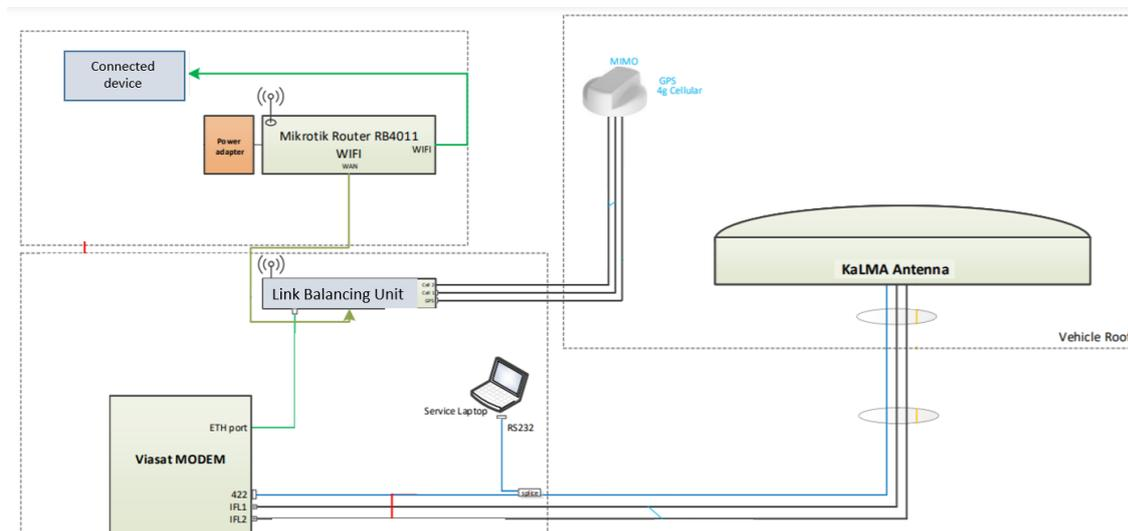
**Figure 13 - Communication hub diagram**
