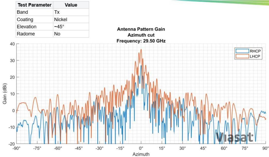
**Figure 44 - Antenna Pattern Gain at 29.5 GHz - Azimuth cut at 45 degree elevation**
