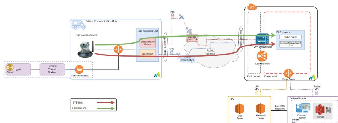
Figure 38 - Diagram for the RT video tests
