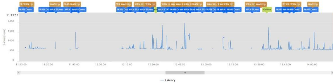
Figure 68 - Timeline graph of the latency on the Satellite link during the long driving test
