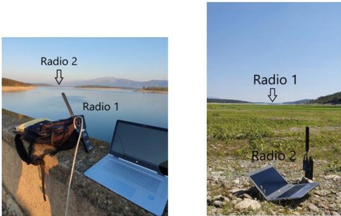
**Figure 86 - Range test at 5.5 km (terrain)**
