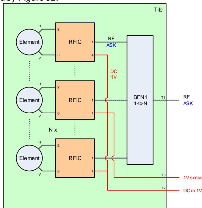
**Figure 32 - Block diagram of the functional tile for N numbers of elements**
