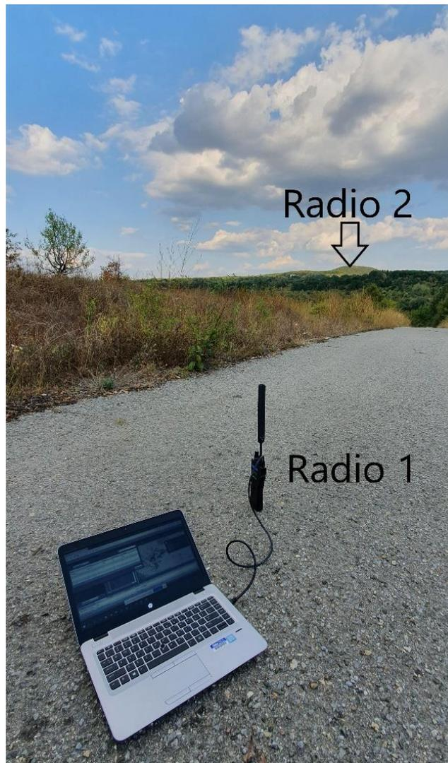
**Figure 83 - Range test at 1.3km (terrain)**
