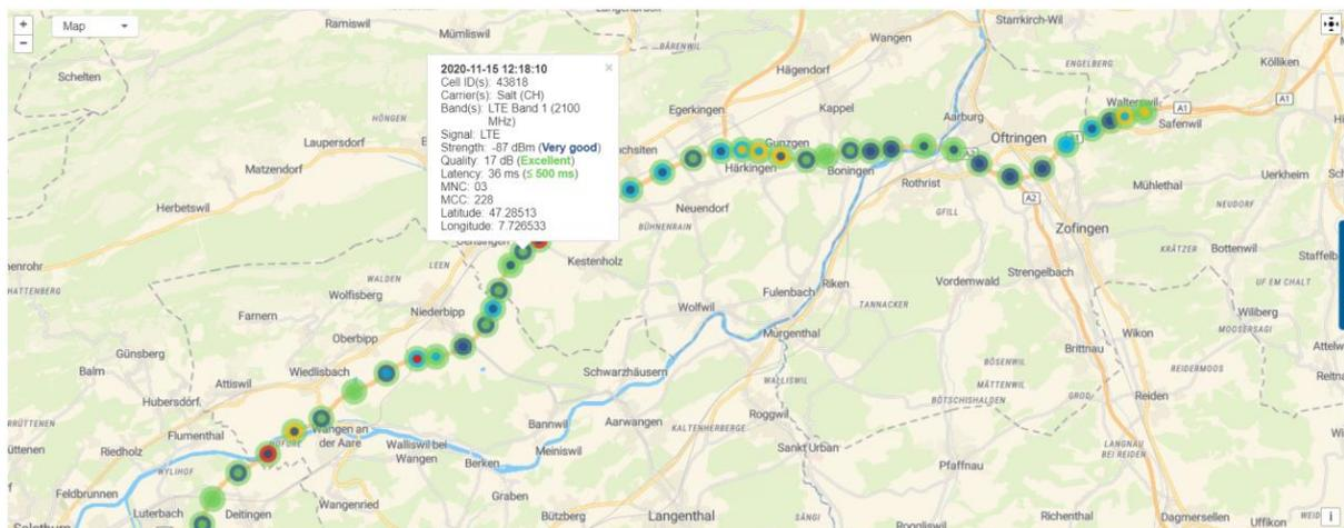
**Figure 72 - Map of the LTE link signal parameters during the failover**
