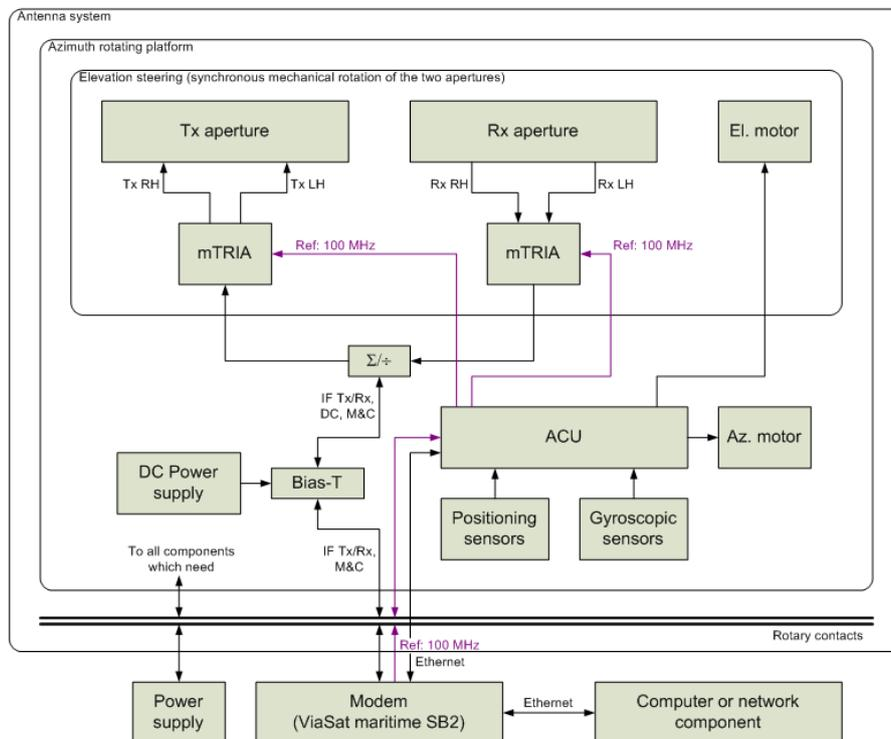
**Figure 29 - Current solution: Directive array on mechanical platform - block diagram**
