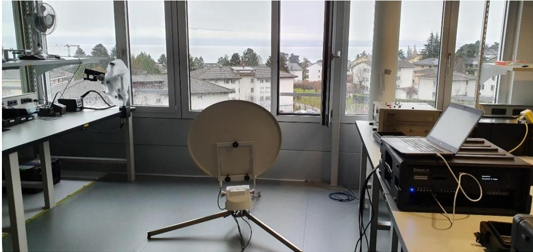
**Figure 21 - Dawson SC Zero 70 KA-SAT antenna system in the Viasat lab (powered off)**
