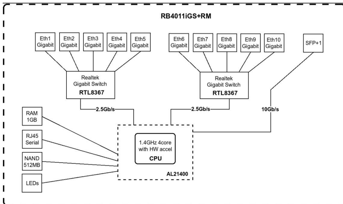
Figure 18 - MikroTik RB4011 schema
