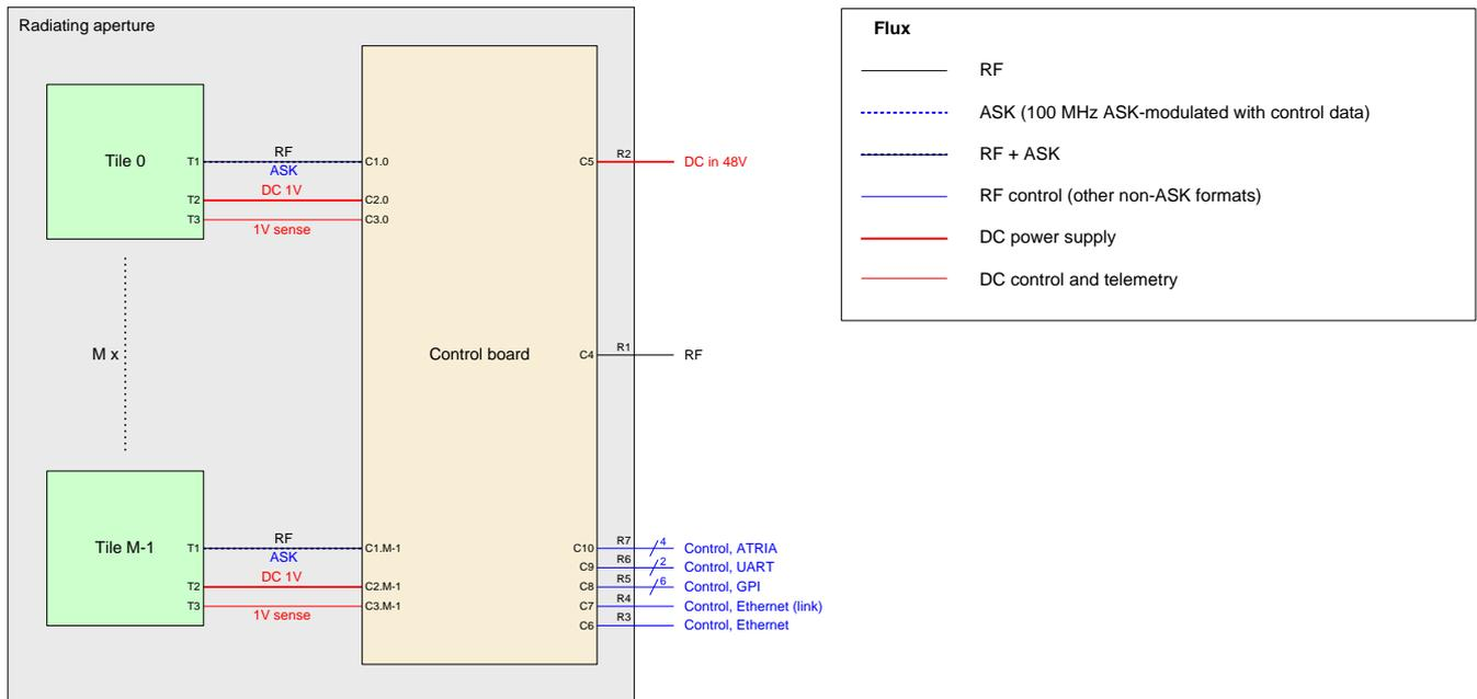
**Figure 31 - Block diagram of the radiating apertures for M tiles used. M is defined according to the performance needed.**
