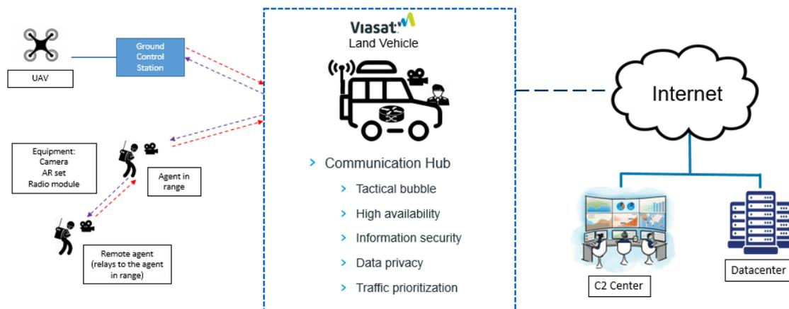
**Figure 6 - ARESIBO Network Architecture schema**
