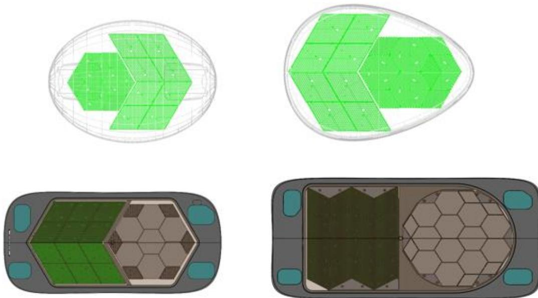
**Figure 34 - Modular approach for phased antenna arrays: using the same tiles (hexagonal for Tx and rhomboidal for Rx) to achieve desired size and performance for various markets and applications.**
