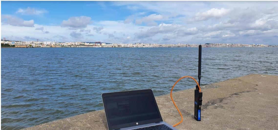
**Figure 97 - Range test at 2.3 km (terrain)**
