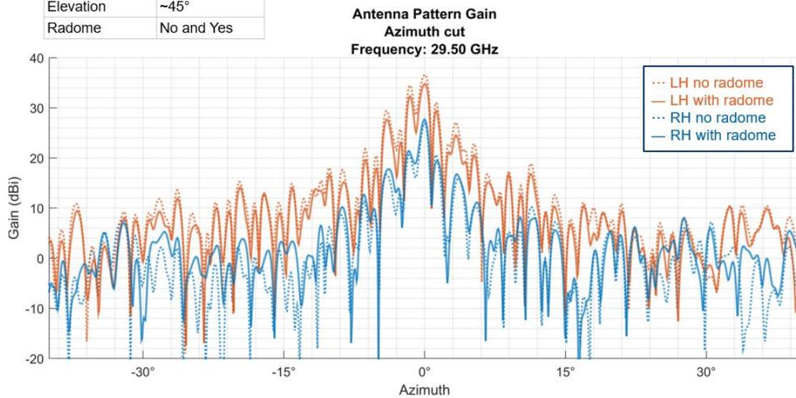
**Figure 52 - Evaluation of the effect of the radome on the Antenna Pattern Gain - Azimuth cut at 29.5 GHz**
