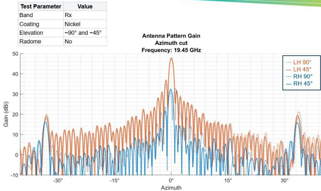
**Figure 46 - Comparison of the Antenna Pattern Gain - Azimuth cut at elevation of 45 and 90 degrees at 19.45 GHz**
