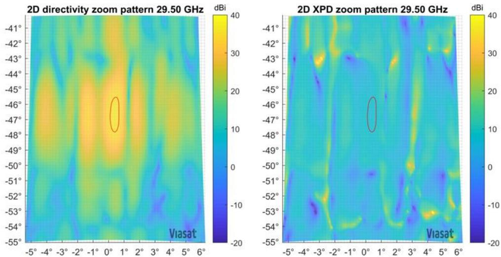
**Figure 56 - Antenna pattern main beam detail at 29.5 GHz at 45 degree elevation with radome**
