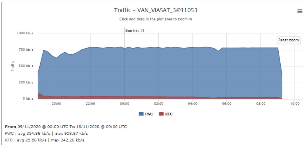
**Figure 76 - Download data rate on the satellite link during the long activity test**
