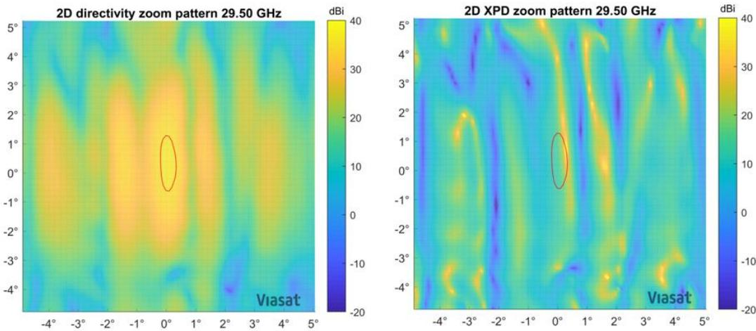
**Figure 54 - Antenna pattern main beam detail at 29.5 GHz at 90 degree elevation**
