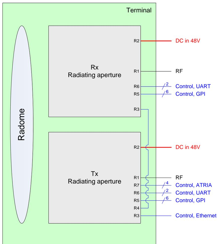
**Figure 30 - High level block diagram of the phased array antenna terminal.**
