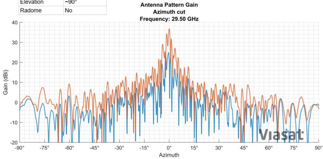
**Figure 42 - Antenna Pattern Gain at 29.5 GHz - Azimuth cut at 90 degree elevation**
