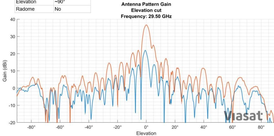
**Figure 43 - Antenna Pattern Gain at 29.5 GHz - Elevation cut at 90 degree elevation**
