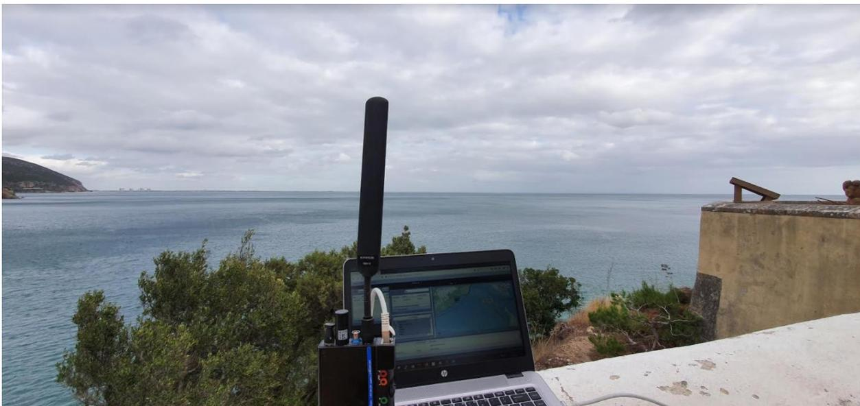
**Figure 104 - Range test at 10km (terrain)**
