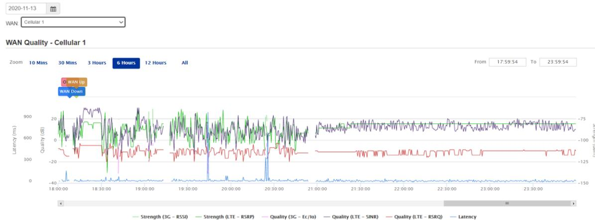
**Figure 64 - Timeline graph of the LTE signal parameters**
