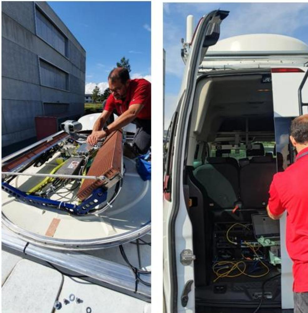
**Figure 24 - KaLMA antenna mounted on the roof of the Viasat Land Vehicle**
