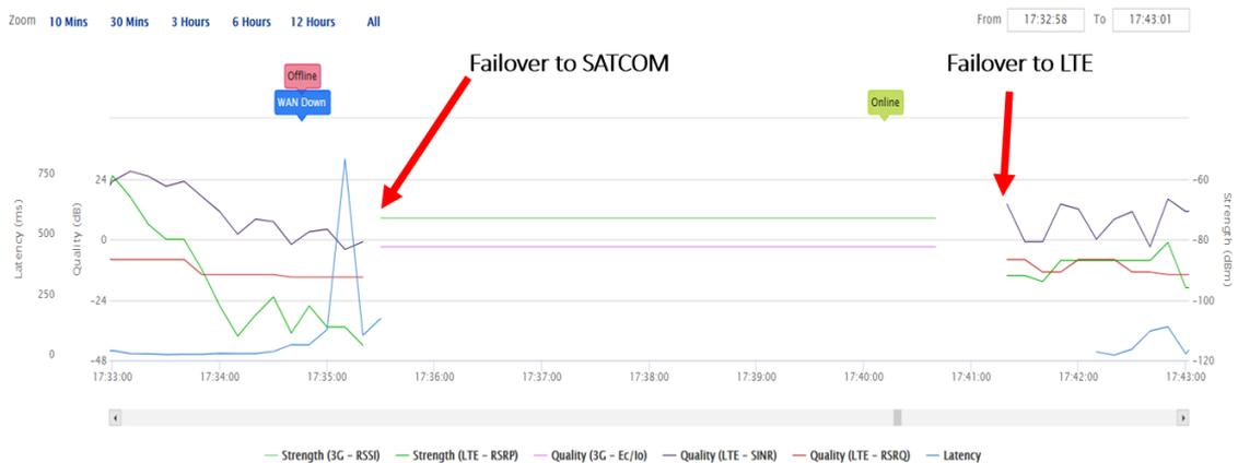
**Figure 65 - Timeline graph of the LTE signal drop**
