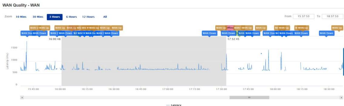
Figure 70 - Timeline graph of the satellite link latency during the deployment test
