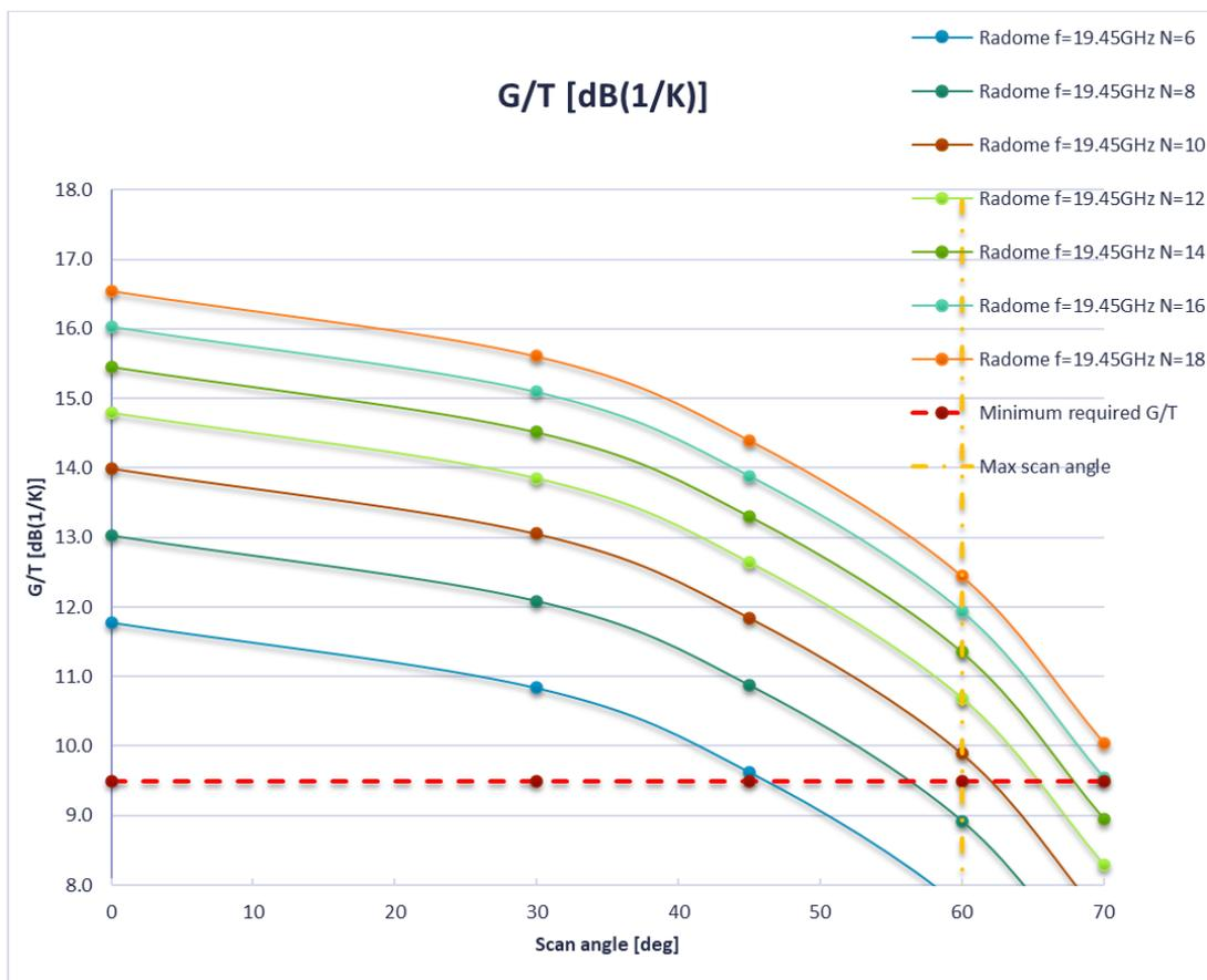
**Figure 35 - Receive aperture performance depending on the number of tiles used. In the example given, if we want to have Gain over Temperature at least 9.5dB/K and to be able to scan down to 60 degrees, we need to combine 10 Receive tiles for the antenna.**
