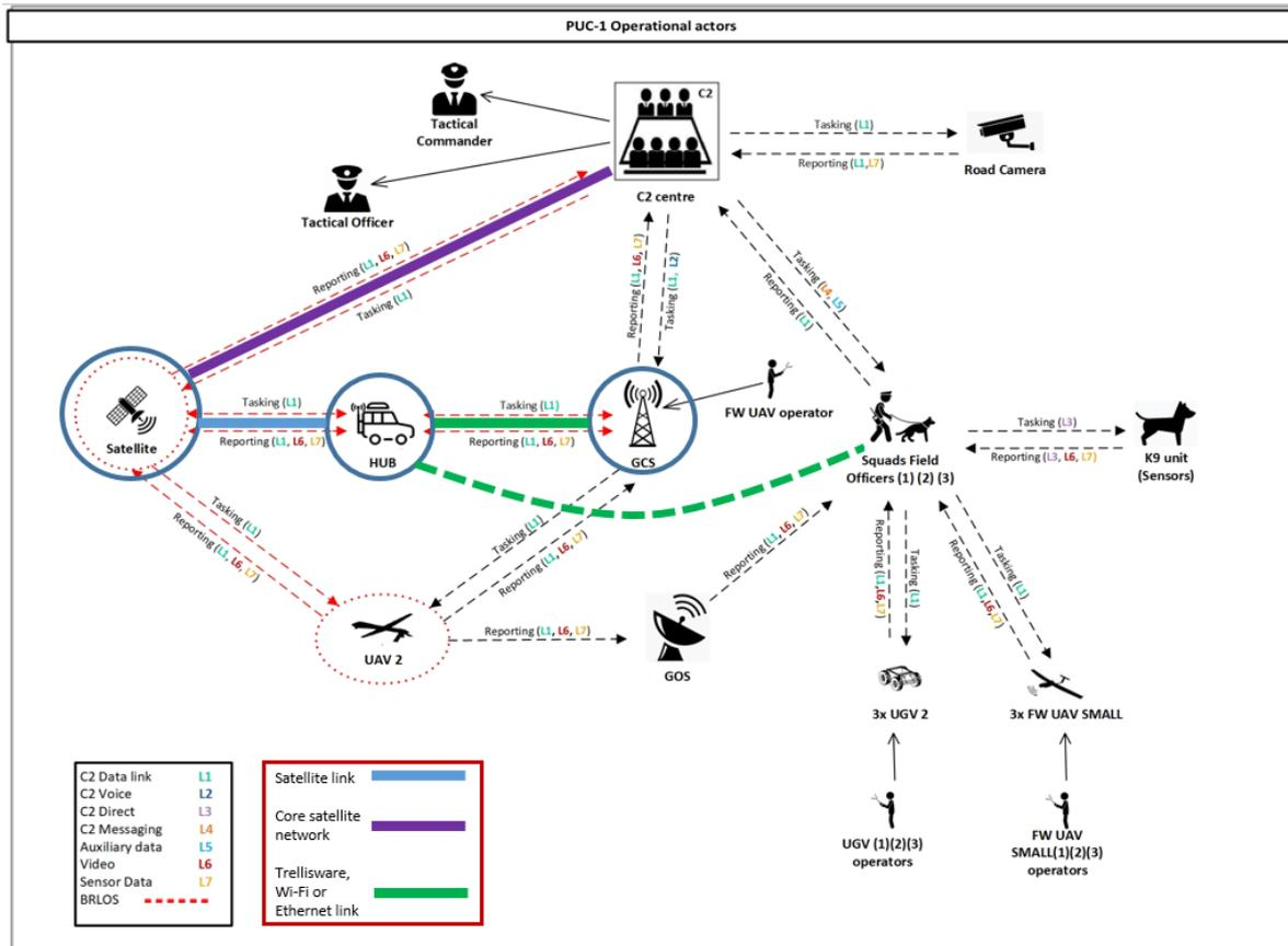
Figure 5 - Links provided by Viasat for PUC 1 with communication hub
