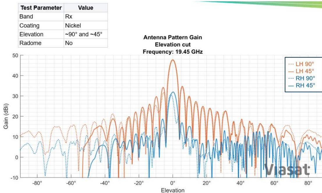
**Figure 47 - Comparison of the Antenna Pattern Gain - Elevation cut at elevation of 45 and 90 degrees at 19.45 GHz**
